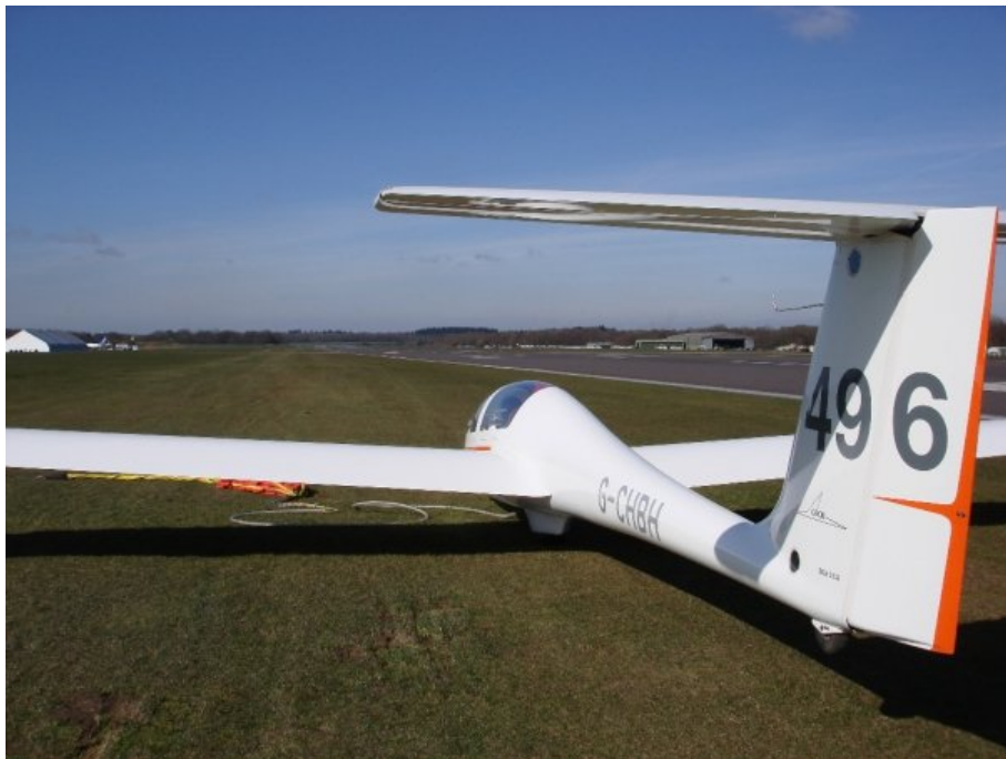
Figure 2: 496 being readied for launch off the winch. The cable will be pulled in and accelerate the glider to 60mph in under 3 seconds, and the glider will then climb up to an altitude of around 1500ft.
